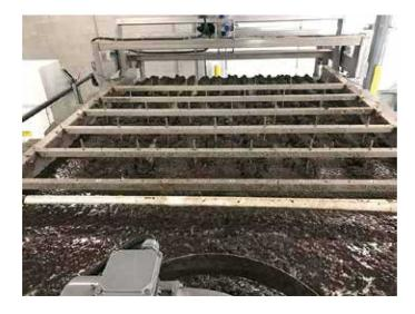
Compactors (OSC7C). Positioned at the inlet of the plant, the screens compact, wash, and lift debris to a convenient height for ease of disposal. These units are provided with perforation size of 6mm for municipal wastewater. The system is stainless steel (AISI 304 or AISI 316) and can be mounted at an angle in a channel, in a tank, or supplied for vertical installation.
