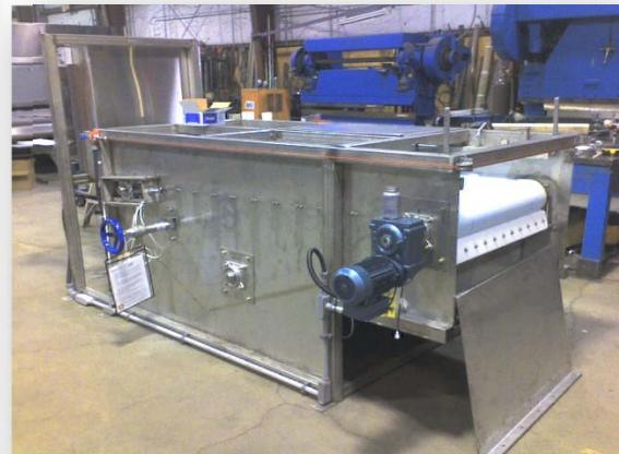
If you're looking for an economical and simple solution to your sludge thickening needs, you'll find an answer in the *OR-TEC Belt Thickener System*. The system is designed with ease of operation, low maintenance, cost effectiveness and thickening efficiency in mind. Its robust frame is constructed of stainless steel and can be trailer mounted for multiple site operation. Available in 0.5, 1.0, 1.5 and 2.0 meter capacities.
