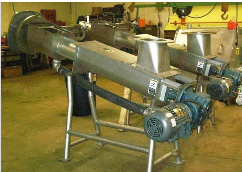
OR-TEC Compactors with back pressure plate discharge
