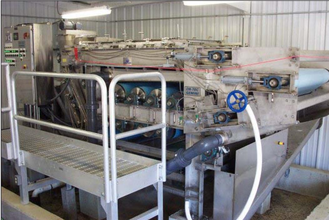
The OR-TEC Gemini Series Belt Press is a double belt system ideal for the medium to large size W.W.T.P. This press combines a gravity drainage zone, a low pressure zone and high pressure shear zone to provide a large dry solids throughput and an excellent final cake. The system can be customized to the clients needs with a full range of ancillary equipment from sludge pumping to dry cake conveying
